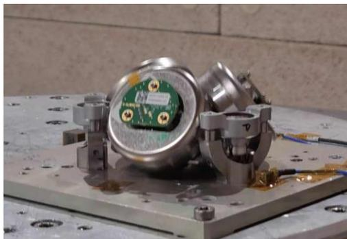
**Figure 5. Photograph of the Sensor Pyramid Mounted on its Set of Dampers for the Test Campaign in Vibrations.**
