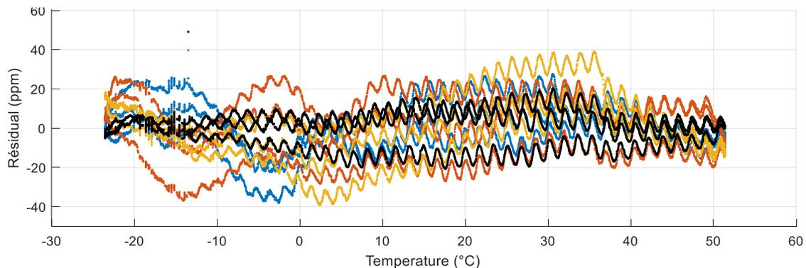
**Figure 3. FOG Scale Factor Residue after Thermal Modeling.**
