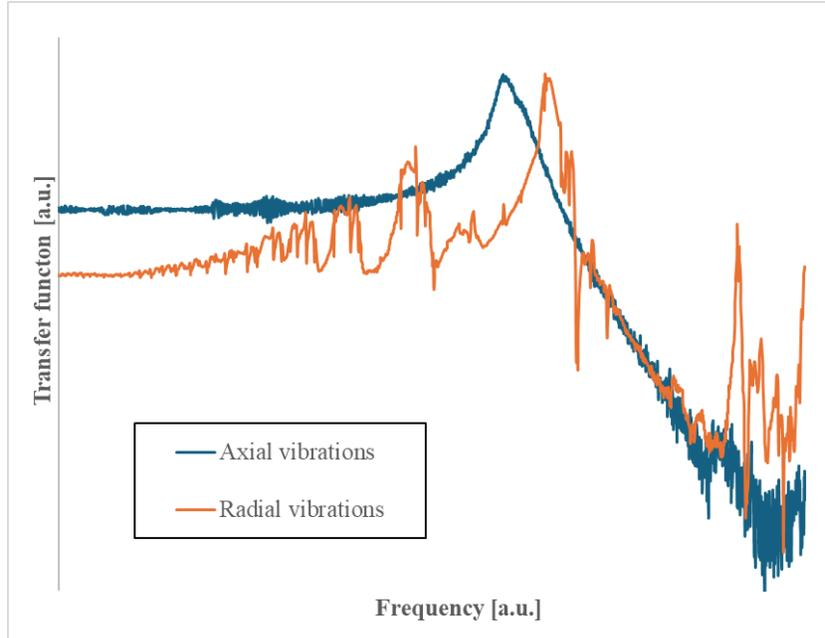
**Figure 7. Mechanical Transfer Functions of the Damper Set Measured during Sinusoidal Vibrations at 0.5g. The Damper Set was Mounted with the Sensor Pyramid for the Test. Scales and Units are Deliberately not Displayed.**
