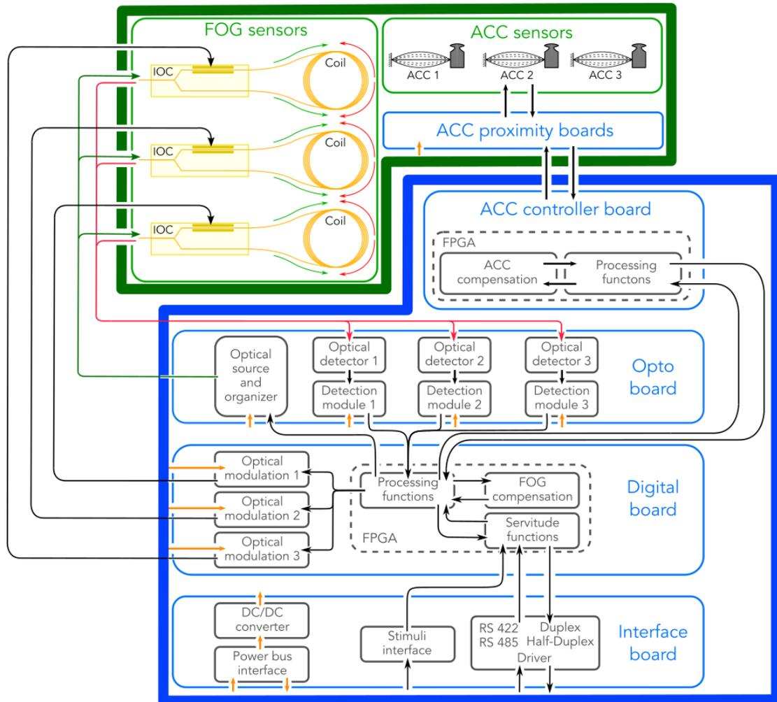
**Figure 1. EURISA IMU Preliminary Architecture Represented as a Block Diagram. Each Blue (Electronic Boards) and Green (Sensors) blocks are Physical Parts. Large green and blue boxes respectively represent the damped pyramid and the electrical stack. Orange Arrows: Power Supply; Green/Red Arrows: in/out Light; Black Arrows: Signal Exchanges.**
