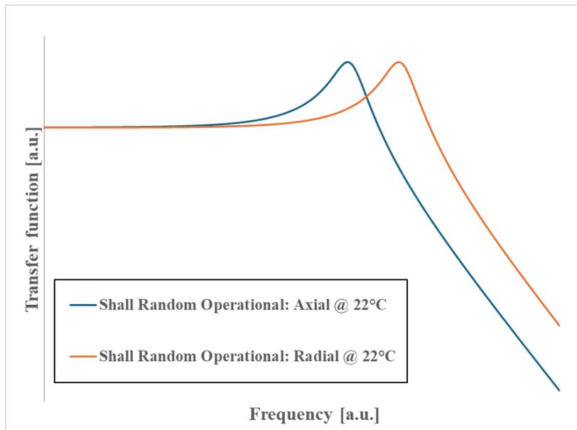
**Figure 6. Theoretical Mechanical Transfer Function of the Dampers in Axial and Radial Vibrations. Scales and Units are Deliberately not Displayed.**
