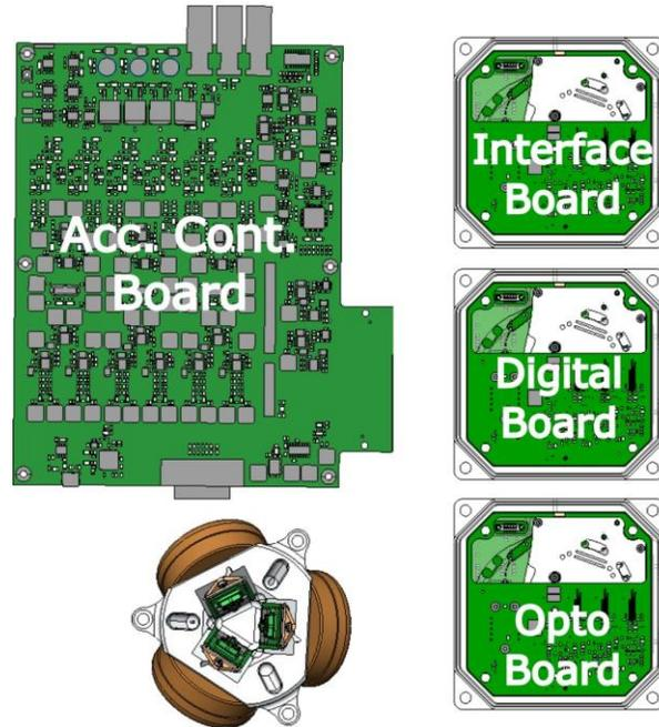
**Figure 8. Schematic of the Flat IMU Including the 3 FOG and 3 Accelerometers Mounted on a Pyramid (bottom left), the Accelerometer Controller Board (Acc. Cont. Board), the Interface Board, the Digital Board and the Opto Board. The Different Components are Connected by Optical and Electrical Wires.**
